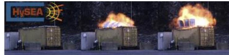
Figure 2: Experimental results of a vented hydrogen deflagration in a 20-foot ISO container (HySEA project, test 61). Comparison with blind-prediction study benchmarks (Skjold et al., 2019).
