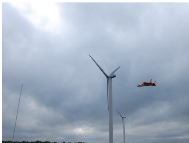
Figure 1: The SUMO system during the initialization before start (left). The 5-hole turbulence measurement probe is the grey tube mounted on the nose of the airframe. The picture on the right shows SUMO in operation in front of two of the NORDEX N80 2.5 MW test turbines at the ECN test site Wieringermeer. The 108 m meteorological mast can be seen in the lower left corner of this picture.
