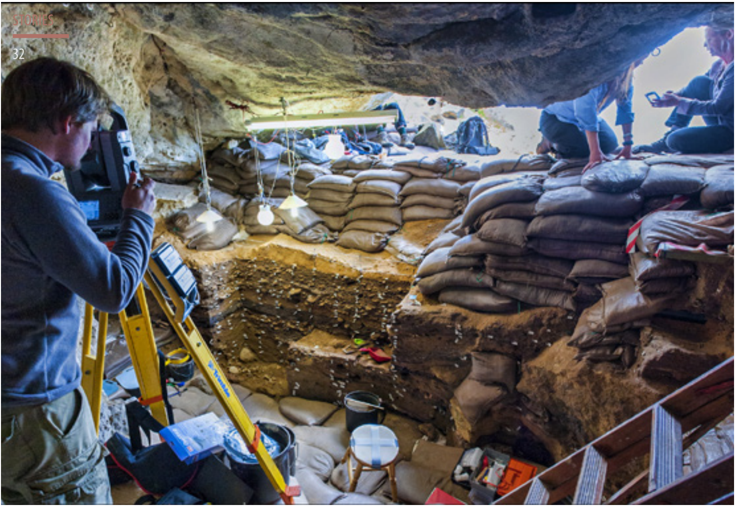
Magnus Haaland recording exact position of samples with a total station in Blombos Cave.
