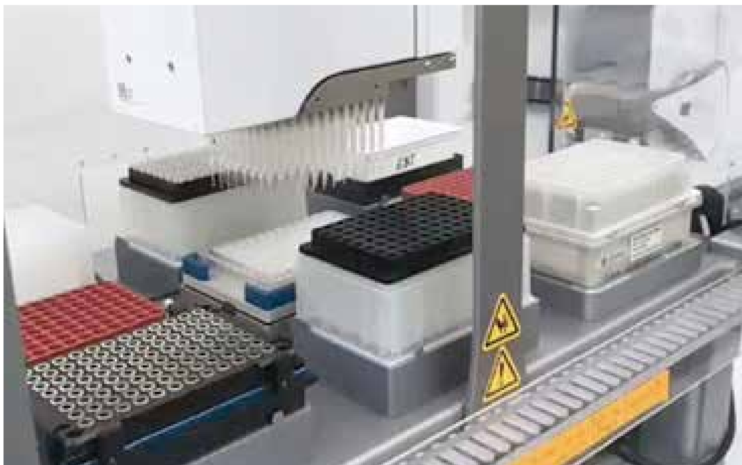
Automated liquid handling system (Bravo NGS workstation, Agilent Technologies) used for preparing ancient DNA from sediments or skeletal remains for sequencing.
