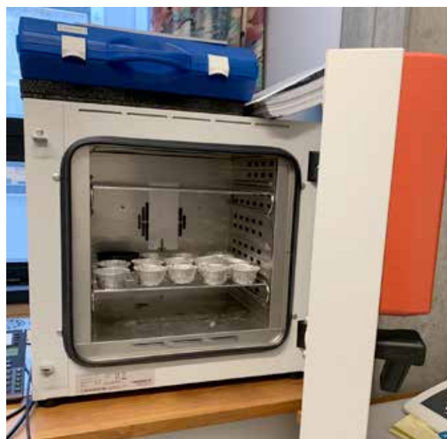
Laboratory setup before heating ostrich eggshells in a laboratory furnace
